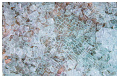
If toughened glass breaks, it shatters into relatively harmless small particles
